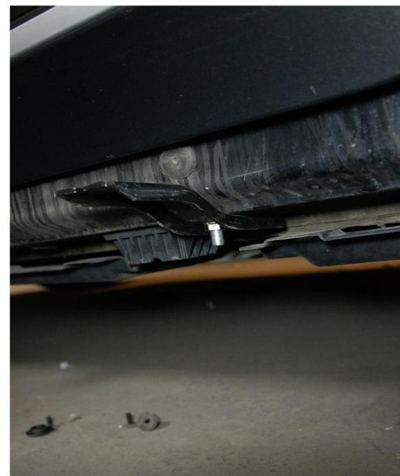
**C –** Put the item no 2 into the hole below the side step and fix the item no 3 with a screw on the side of the car. Link the item no 1 with the items no 2 and 3. After that, use 2 screw nuts to tighten the screws below.
