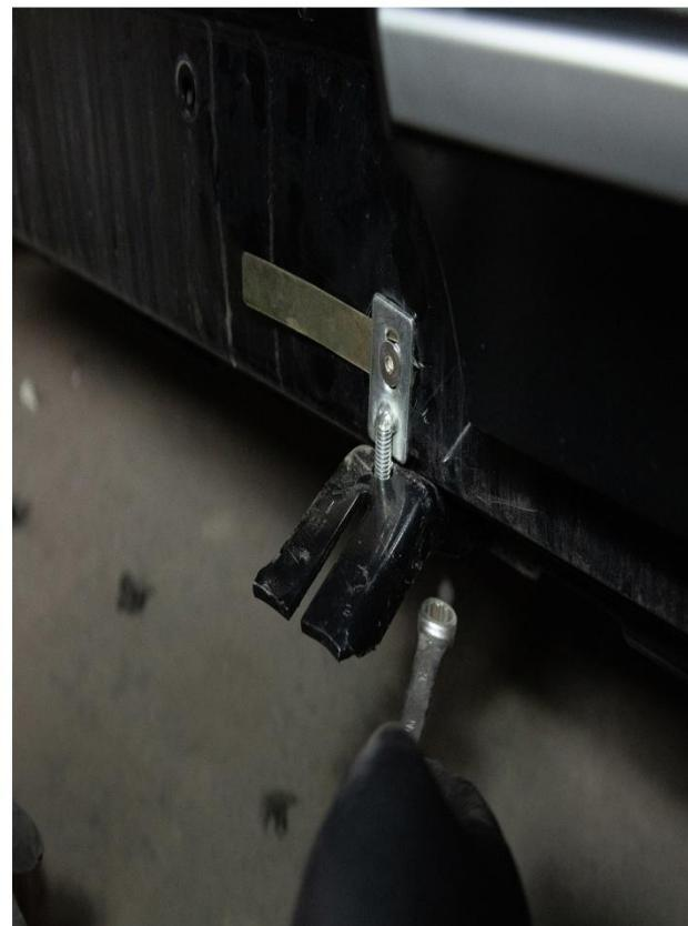
**B)** — Put the item no 2 into the hole below the side step and link it with the item no 1.
